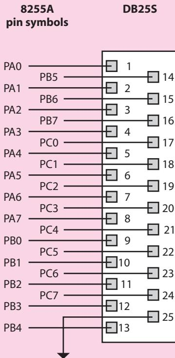
**Port A, (8255A Pins 0-3):** Lower nibble of an 8-bit data output latch/buffer and an 8-bit data input latch.
